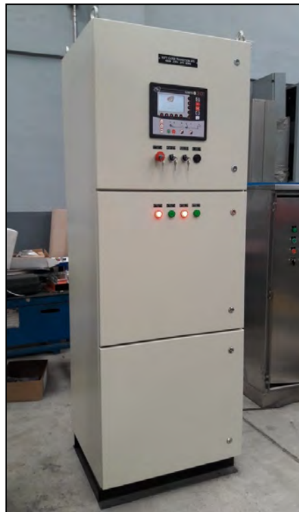
LV SOFT CLOSE TRANSITION ATS for MAYNILAD NOVALICHES PS & RESERVOIR
